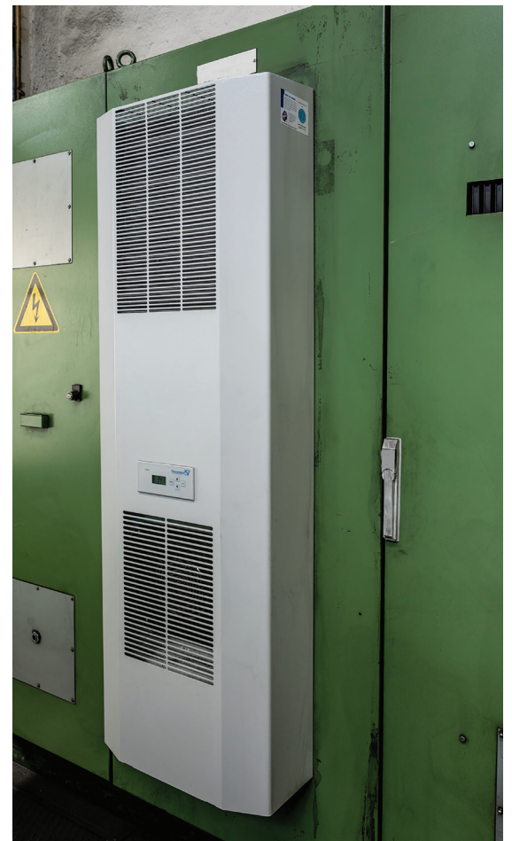
Picture above: The operating unit (Premium Controller), specially developed for the X-series, enables communication between the cooling unit and the machine control system, as well as integration into modern production processes.
