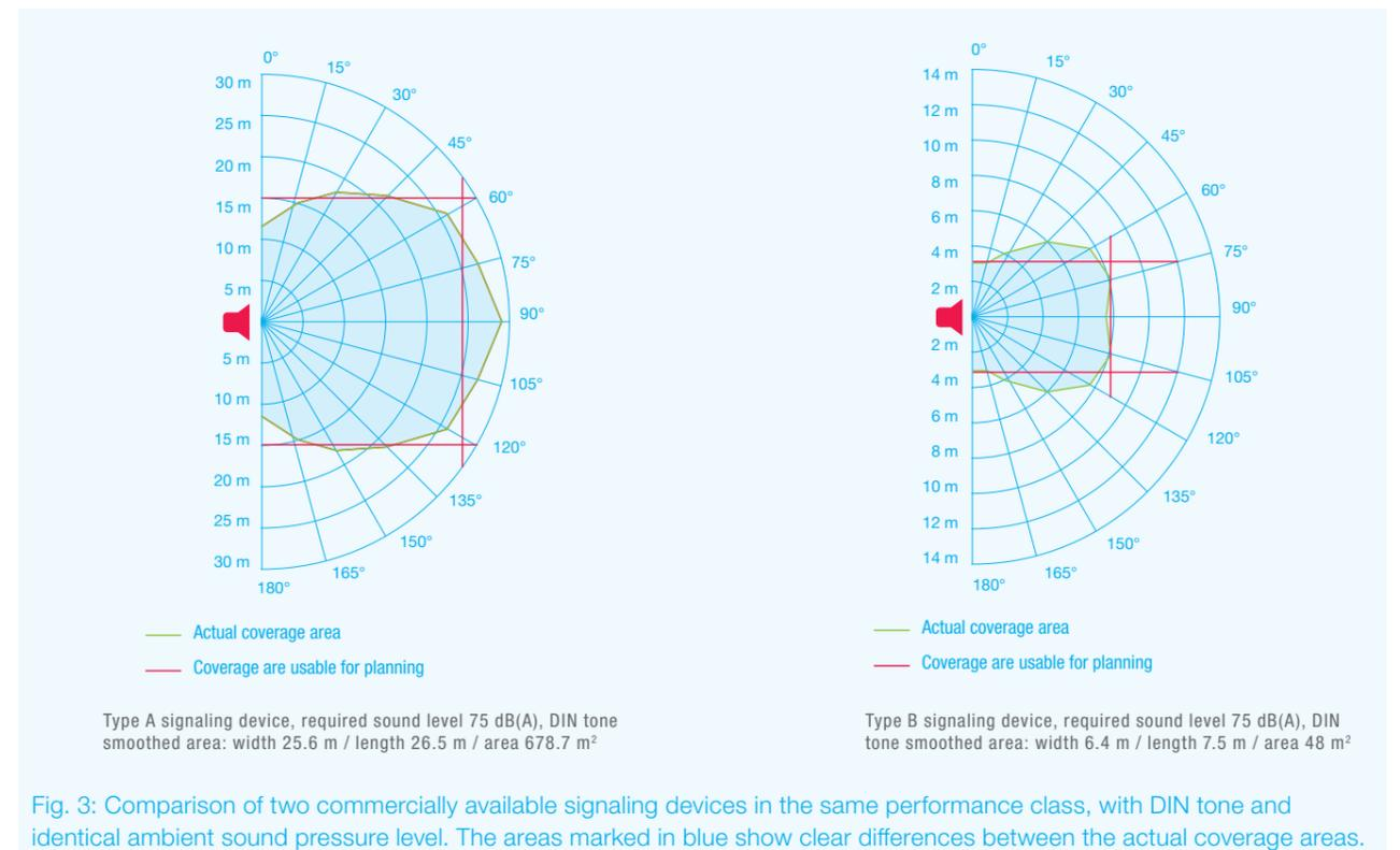
Fig. 3: Comparison of two commercially available signaling devices in the same performance class, with DIN tone and identical ambient sound pressure level. The areas marked in blue show clear differences between the actual coverage areas.
