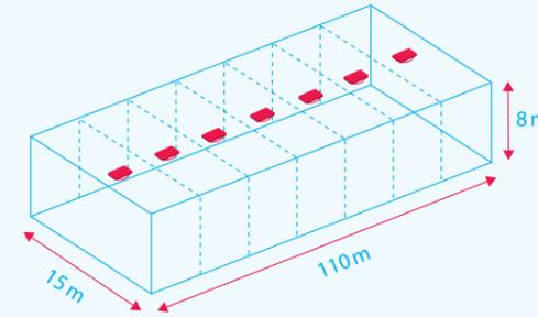
Fig. 11: Seven devices in the light colour "red" are needed to provide an alert throughout the area specified.
