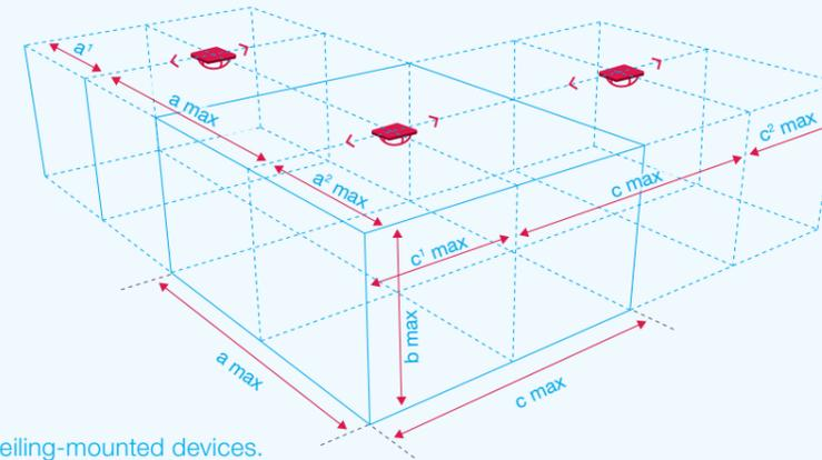
Fig. 7: Ceiling-mounted devices.
