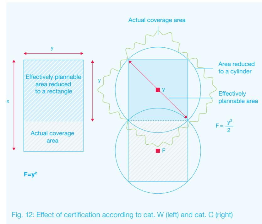
Fig. 12: Effect of certification according to cat. W (left) and cat. C (right)
