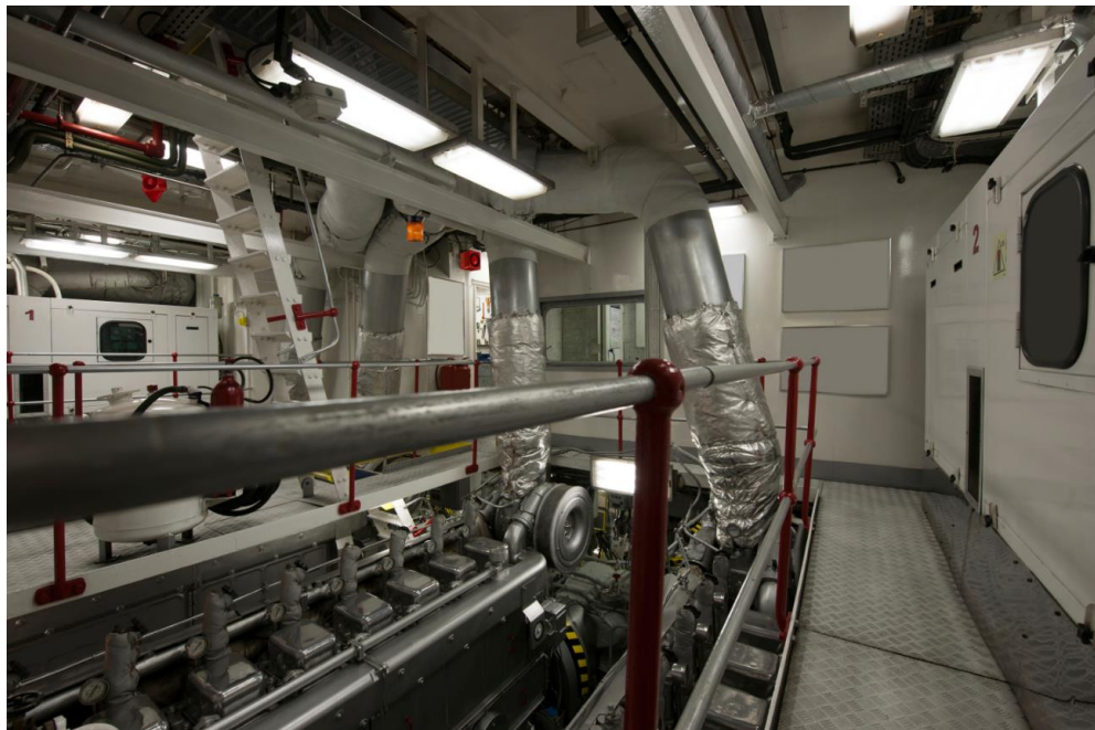
001484_Picture1: A yacht machine room with Pfannenberg products: PATROL series flashing sounders, PMF all-round light and a powerful DS series sounder.
