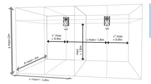
Signaling ranges of the PATROL flashing light sounder PA X 1-05, 24 V DC, red lens, using the example of **wall mounting.**
