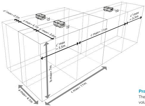
Signaling ranges of the PATROL flashing light sounder PA X 1-05, 24 V DC, clear lens, using the example of **ceiling mounting.**
