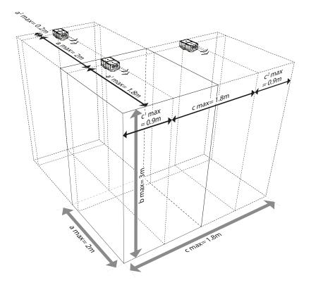
Signaling ranges of the PATROL flashing light sounder PA X 1-05, 24 V DC, red lens, using the example of **ceiling mounting.**
