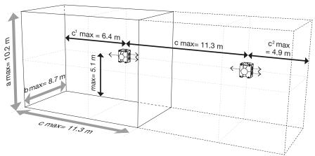
Signaling ranges of the PYRA flashing light PY X-S, 24 V DC, clear lens, using the example of wall mounting.
