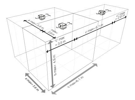
Signaling ranges of the PYRA flashing light PY X-S, 24 V DC, red lens, using the example of **ceiling mounting.**
