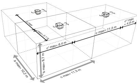
Signaling ranges of the PYRA flashing light PY X-S, 24 V DC, clear lens, using the example of **ceiling mounting.**
