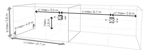
Signaling ranges of the PYRA flashing light PY X-S, 24 V DC, red lens, using the example of **wall mounting.**
