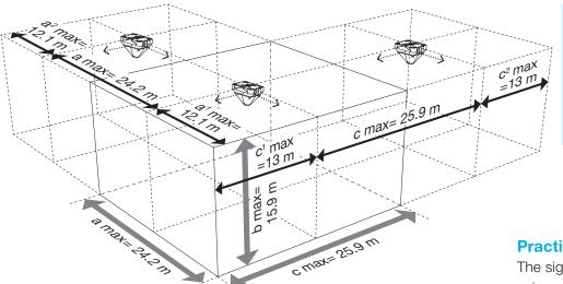
Signaling ranges of the PYRA flashing light PY X-L-15-CPR, 24 V DC, clear lens, using the example of
