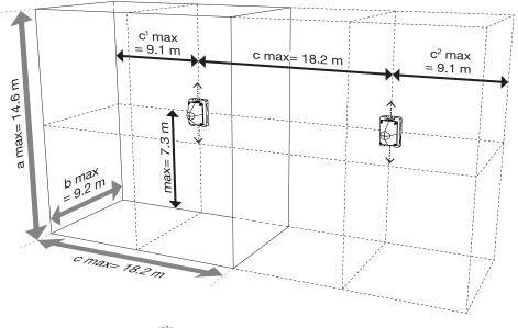
Signaling ranges of the PYRA flashing light PY X-L-15-CPR, 24 V DC, red lens, using the example of **wall mounting**
