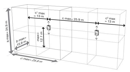
Signaling ranges of the PYRA flashing light PY X-L-15-CPR, 24 V DC, clear lens, using the example of wall mounting
