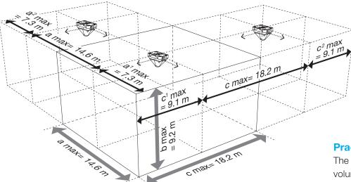
Signaling ranges of the PYRA flashing light PY X-L-15-CPR, 24 V DC, red lens, using the example of **ceiling mounting**
