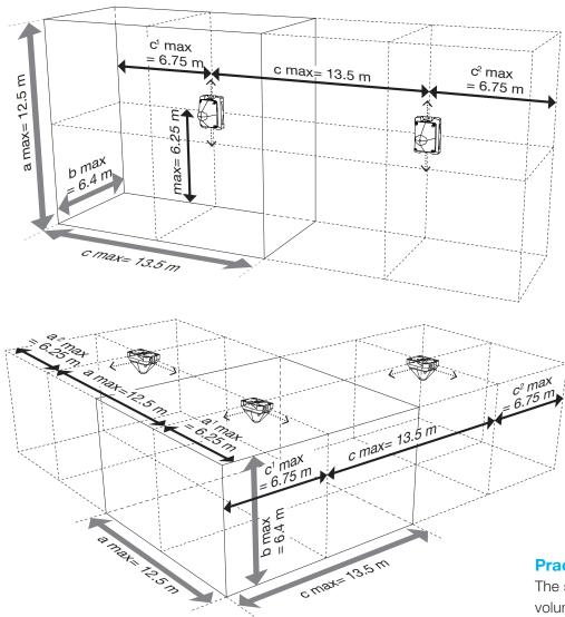
Signaling ranges of the PYRA flashing light PY X-M-05-SSM, 24 V DC, clear lens, using the example of **wall mounting**
