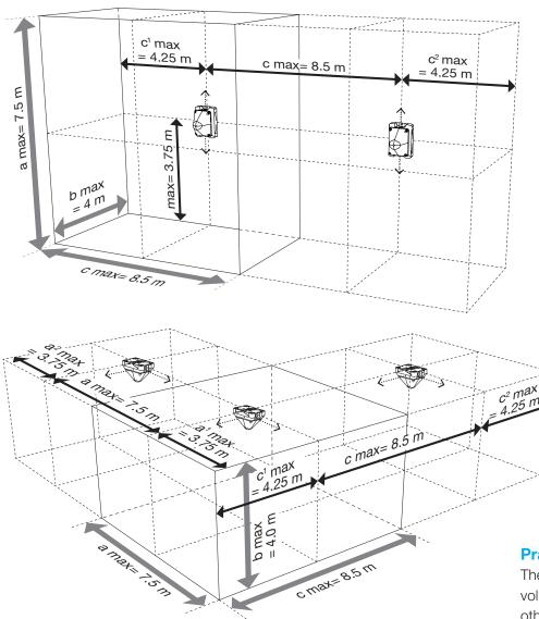
Signaling ranges of the PYRA flashing light PY X-M-05-SSM, 24 V DC, red lens, using the example of **wall mounting**
