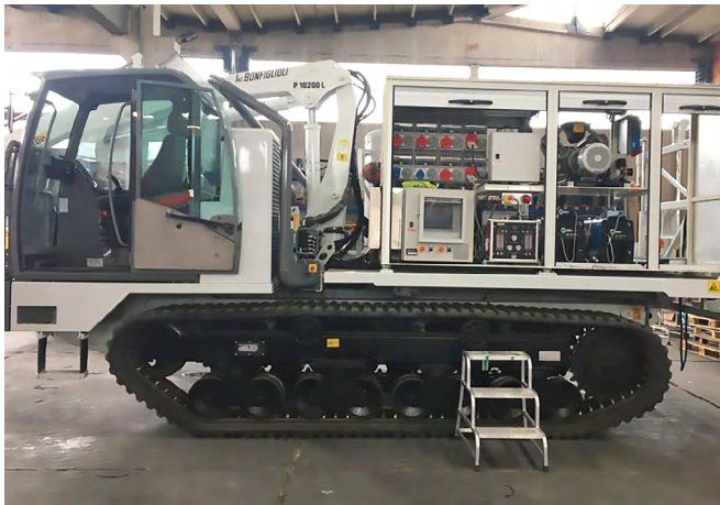
Control cabinet and Pfannenberg cooling unit on a SICIM paywelder machine.
