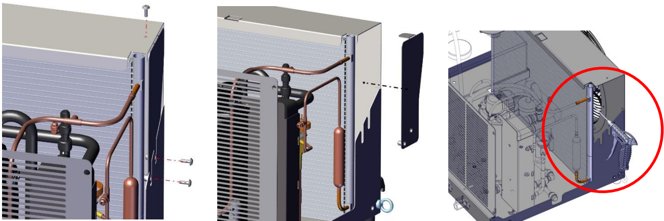
Picture 18 – Condenser cleaning
