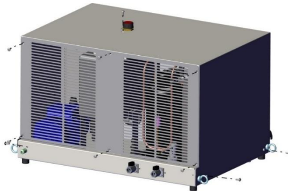
Abbildung 14 - screws to be removed to have access to the chiller
