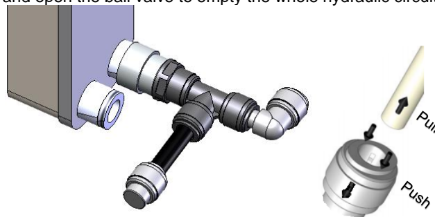
Picture 19 – Chiller draining
